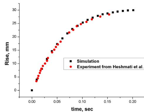
Fig. 8. Capillary rise comparison between experiment and simulation.
