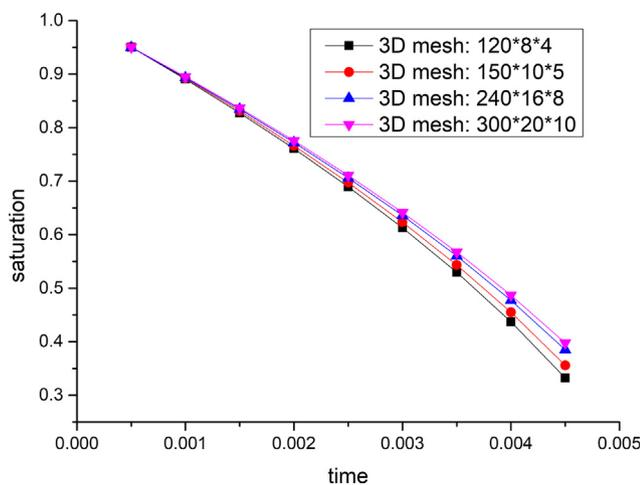
Fig. 4. Mesh independence test for drainage in 3D duct.
