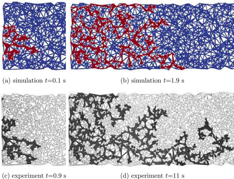
Fig. 10. Comparison between simulation and experiment for micromodel 2.
