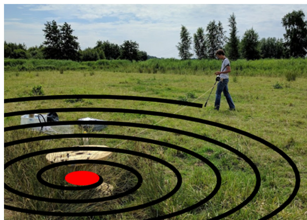
Fig. 2. Photo of the surficial scanning in action. Operator is attached to a wooden cylinder placed on the estimated location of the buried well, as marked with a red dot. The black line schematically shows the remaining path to be walked.
