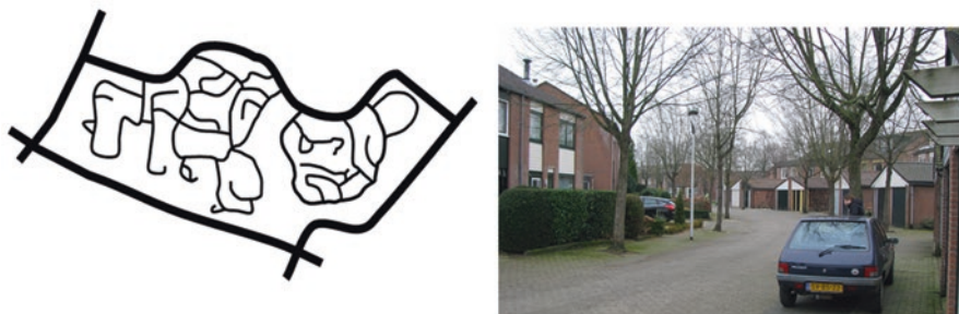
Fig. 19.5 Cauliflower network pattern with winding roads and limited access (left); example of a winding road in a cauliflower neighbourhood (right)
