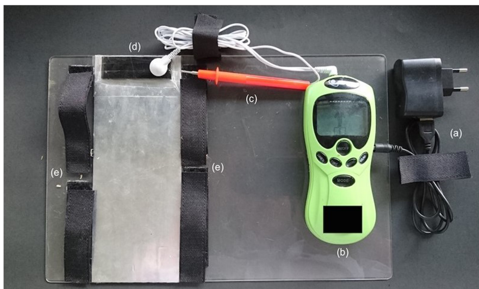
Fig. 1 The device for electrical shock study. The device was set up to deliver an average electric current of 3.161 \pm 0.18 mA, applied to each mouse for 400–600 ms
