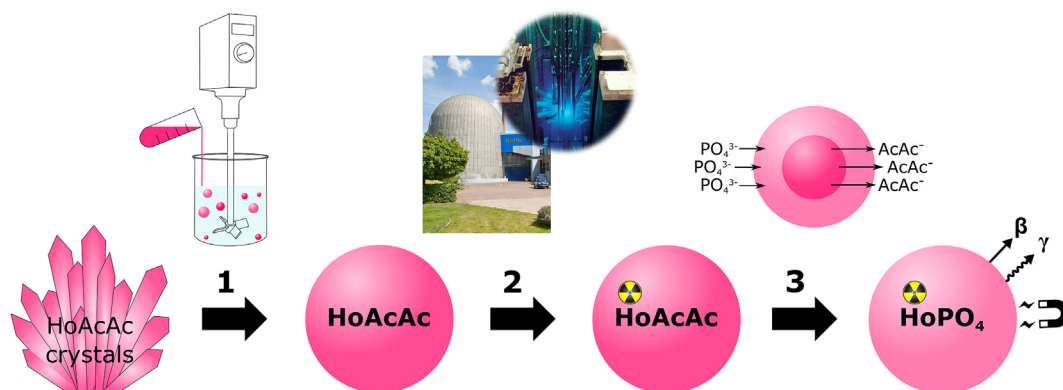
Fig. 1. Schematic overview of the preparation of radioactive holmium phosphate microspheres: (1) holmium acetylacetonate microspheres (HoAcAc-MS) were prepared by dissolution of holmium acetylacetonate crystals in chloroform followed by solvent evaporation. The obtained microspheres were (2) neutron activated in a nuclear research reactor where the ^{165}\text{HoAcAc-MS} were converted into radioactive ^{166}\text{HoAcAc-MS} . Finally, (3) the AcAc ligands were exchanged by phosphate ions by simply incubation of the ^{166}\text{HoAcAc-MS} in a phosphate buffer solution to yield radioactive holmium phosphate microspheres (HoPO 4 -MS).
