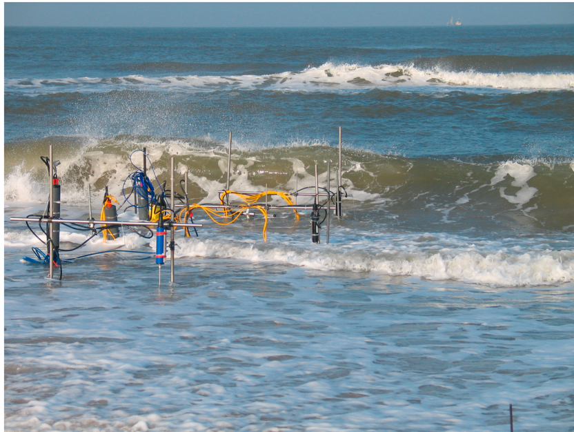
Figure 1. Plunging breaker at the shorebreak at Vejers. Landward of the shorebreak, a surf bore is propagating onshore in the inner surf zone. In the background, an outer breaker zone is located over the inner subtidal bar.
