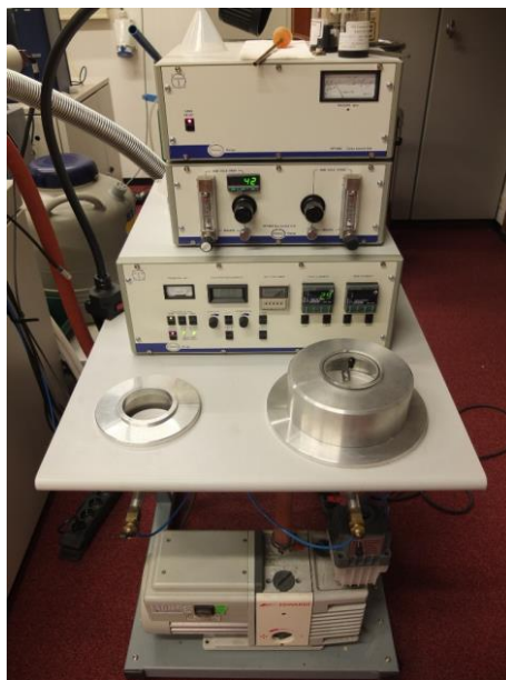
Figure B4: The advanced transfer unit with the temperature regulators for the cryo-stage and the cold trap and an indicator for the SEM chamber pressure. Below is the turbo pump.
