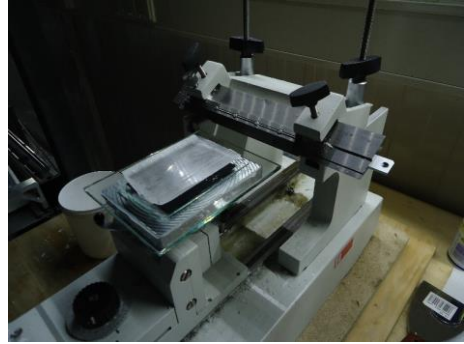
Figure A2: A microtome with a glass plate and an ice core section glued to it with the black cloth between the glass plate and the ice core section.
