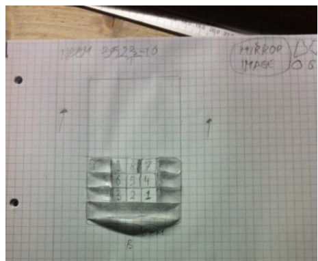
Figure A6: Overview of the location of the EBSD samples in the 90 x 55 mm ice core section.
