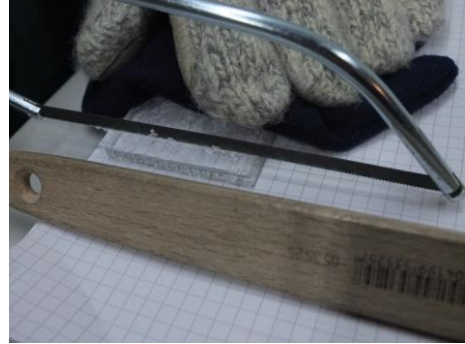
Figure A5: Sawing 8 mm thick bars perpendicular to the core axis.
