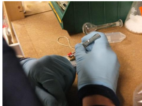
Figure B3: Mounting of the EBSD sample on the stub while holding the EBSD sample in place with a tweezer.
