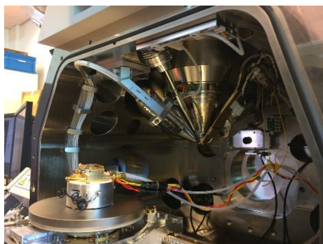
Figure B2: The cryo-stage with the white tubes carrying the cooled nitrogen gas to the cryo-stage and the red and yellow wires for the thermometer. The cold trap is installed next to the pole piece.
