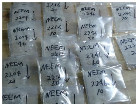
Figure A1: Packed ice core sections (90 x 55 mm) from the NEEM ice core.
