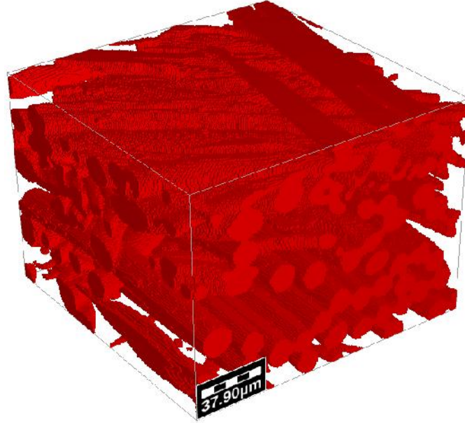
Figure 3.2 Binary three-dimensional domain of fibrous layer
