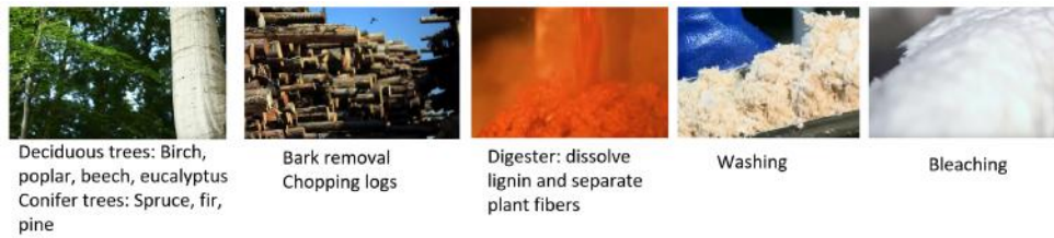
Figure 1.4 Paper manufacturing steps, from tree to white fiber
