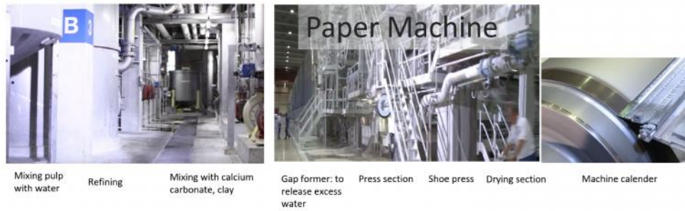
Figure 1.5 Paper manufacturing steps, from white fiber sheets to calendered fibrous layers
