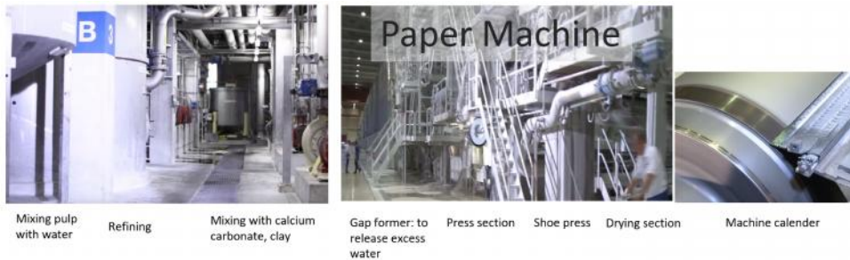
Figure 1.5 shows the processes taking place in a paper machine.
