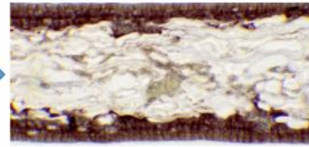
Each side is coated and dried in sequence to create the correct characteristics for each paper grade
