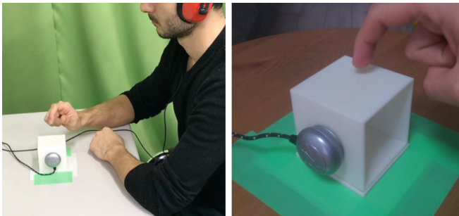
Fig. 2. Setup for experiment 1: (left) Participants tap the top of a solid or hollow cube. There is visually no distinction between the two thicknesses (during the experiment, the opening in the right figure was facing down). The cube is placed in a holder that is firmly attached to a table surface. A piezoelectric sensor is attached to the side of the cube (right) to capture vibrations in the material.
