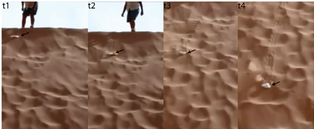
Fig. 25. Sliding sublimating CO 2 ice blocks down dunes as analogues for Martian linear gullies, frames were captured from the video included as Supplementary video 4 in Dinięga et al. (2013) , where a block is released over a 20° slope on Kelso Dunes, California; the person at the dune brink is for scale. Black arrows point to the block at each time step, labelled t1–t4.
