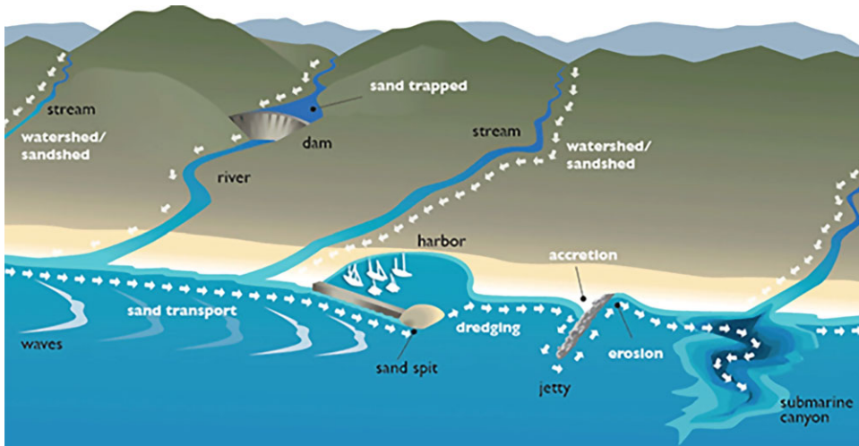
Figure 3.1. Sediment transport along the coastal areas (Source: Dave Hubbard, Monica Pessino, and Molly Thomson; adapted from M. Myers (Explore Beaches, 2017)).
