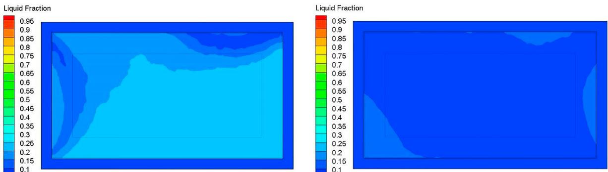
Fig. 5. Liquid fraction contours of (a) the floor PCM plate; and (b) the roof PCM plate at 57600 s.
