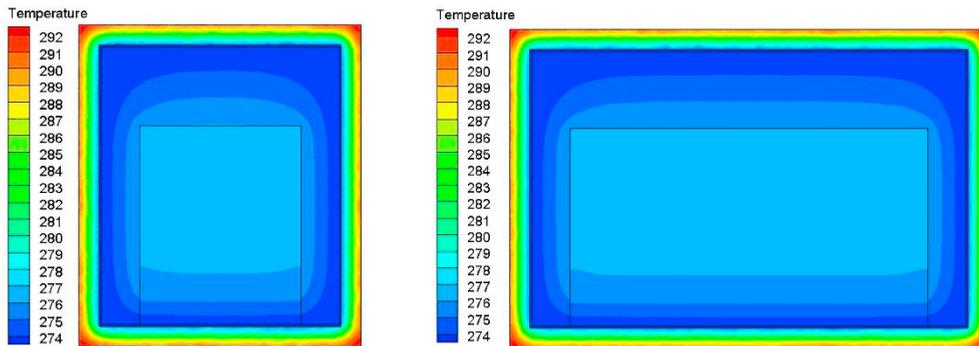
Fig. 4. Temperature contours of (a) the YZ side at  $X=1.2$ ; and (b) the XZ side at  $Y=0.7$  at 57600 s.
