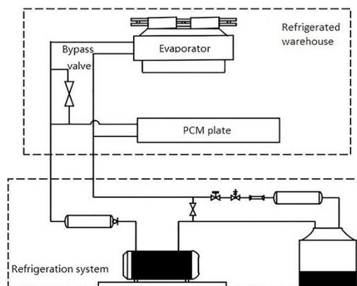
Fig. 1. Schematic diagram of applying latent heat cold storage in a refrigerated warehouse
