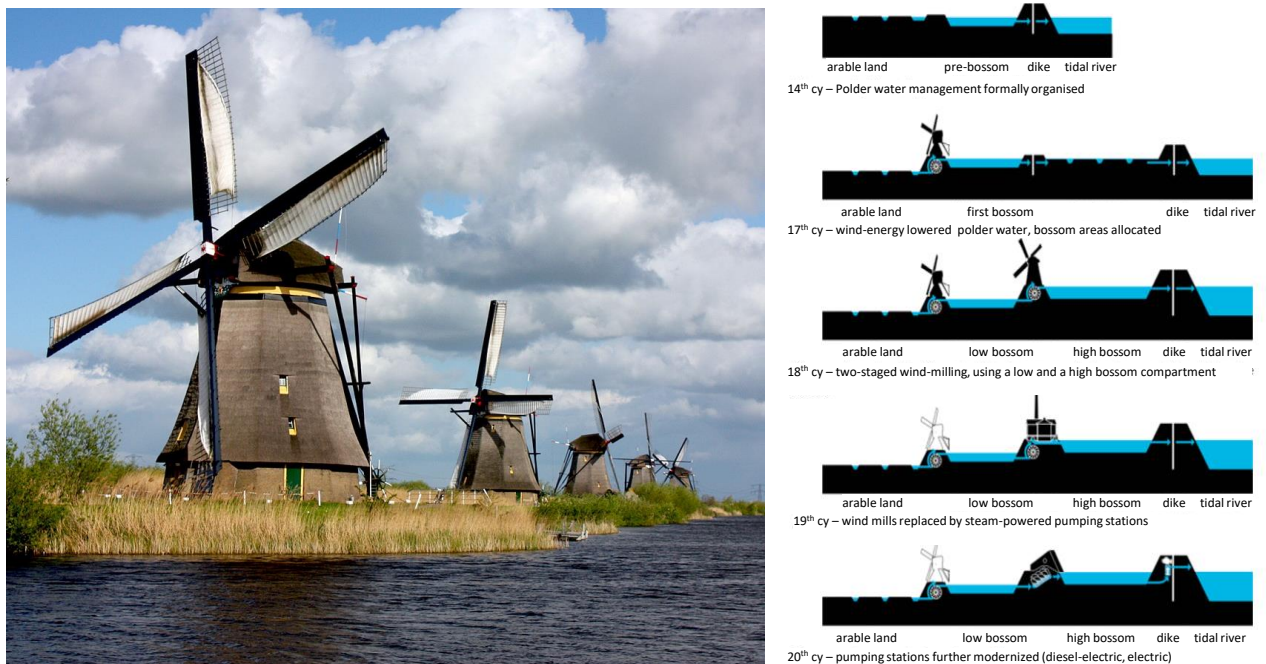
Fig. 4 – a) Series of windmills at ‘Kinderdijk’ (photo: Wikipedia), b) timeline of need for more milling / pumping capacity with aging of the medieval reclamation (Schengenga et al. 2013) . The polder side is behind the wind mills in the photo (left in panel b). The water in front of the mills is the ‘bossom’ (middle of panel b): the polder compartment used to collect the wind-milled waters and route and release them to tidal river and sea (at low tide, free flow).
