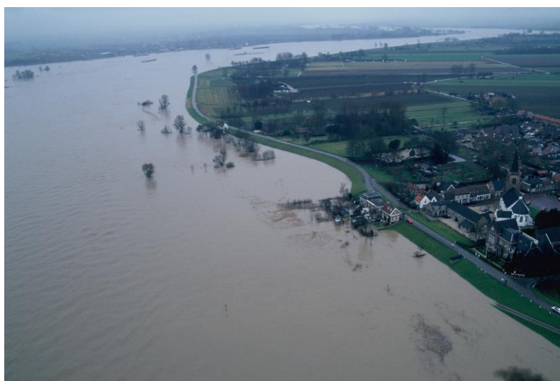
Fig. 2a – The Hagestein weir in the Lek River. River flow is from right to left. The photo shows the weir closed at normal discharge. The weir is opened during river peak discharge. 2b – Inundation of the embanked floodplain of the Lek River in 1993 during peak discharge (source: RWS).
