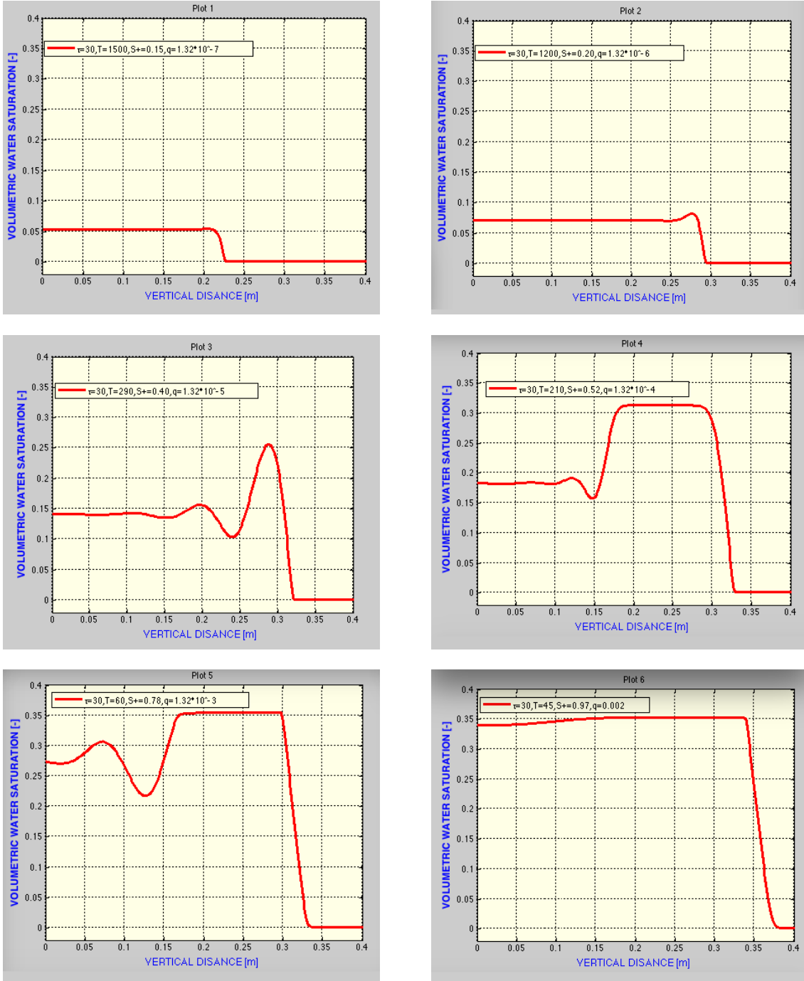
Figure 5.2: Numerical simulation results of DiCarlo's experiments with method of lines in combination with IMEX.
