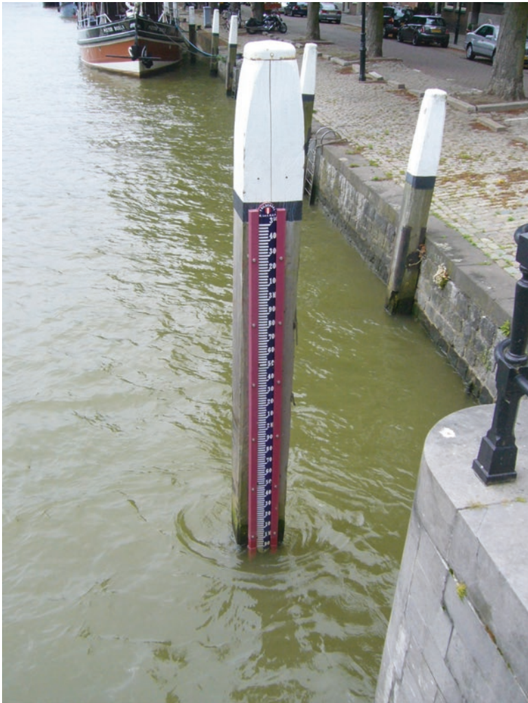
Fig. 4.1 Water level measurement in Dordrecht, the Netherlands
