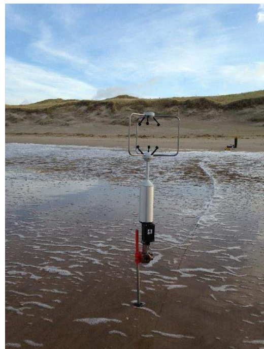
Figure 1. An ultrasonic anemometer in front of the high and steep foredune at Egmond aan Zee, the Netherlands.
