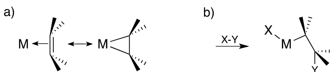
Figure 2. a) Resonance extremes of an alkene binding to a metal center, left: side-on adduct, right: metallacyclopropane adduct. b) Addition of a substrate X–Y to this bond, altering the binding mode to form a \sigma -bond with one of the olefinic carbons.
