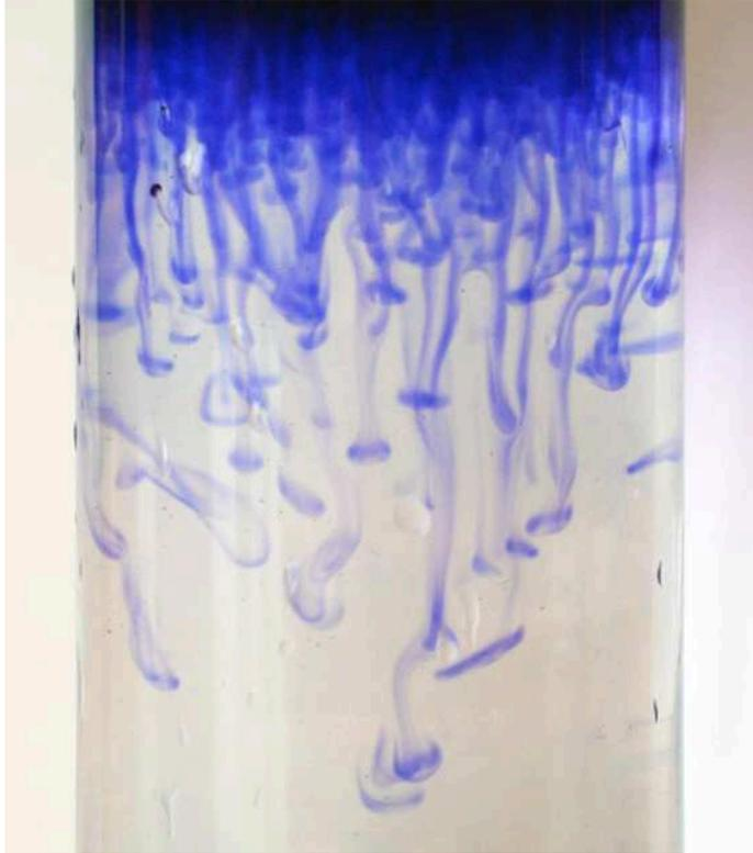
Figure 1.5: Thermohaline mixing in a glass of water. A layer of warm, salty water colored with a dye, is standing on top of a layer of fresh, cold water. While losing their heat content, finger-like structures slowly make their way to the bottom of the glass. Also shear develops at the finger's top, resulting in Kelvin-Helmoltz instability.
