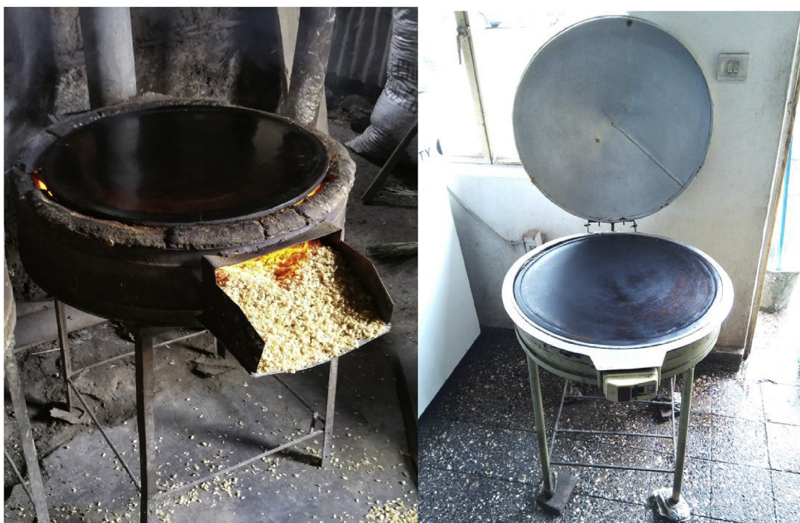
Fig. 1. Left—a traditional biomass powered cookstove (photo credit co-author Hugo van der. Zwaag) and right — an electric mitad (photo credit Energypedia, creative commons licensing (File, 2017)).
