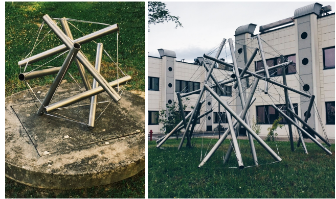
Fig. 5. Two physical tensegrity models constructed from our designs using 60 mm wide stainless steel tubes and 4 mm wide steel cables. Left: a spherical design featuring 7 struts, which is a non-trivial asymmetric variation of the popular icosahedron-based 6 struts tensegrity. Right: realization of the design shown in Figure 7-(b); see also Figure 14 and the attached video.
