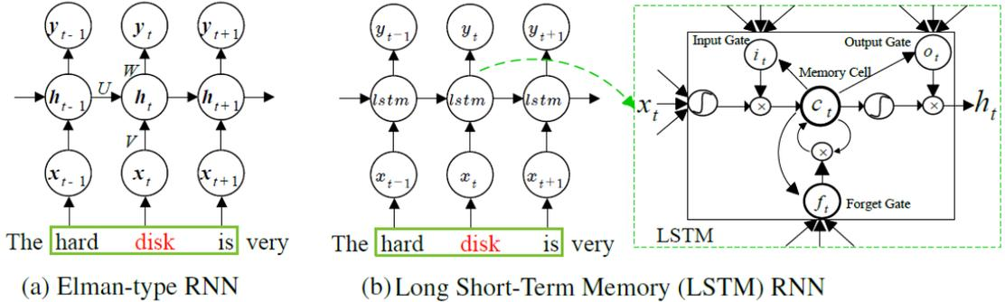
Figure 10: Elman-type and LSTM RNNs with an input layer, a hidden layer and an output layer. [29]
