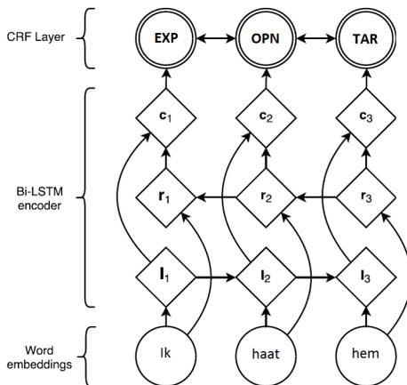
Figure 12: Diagram of the network architecture used for expresser and target identification. Word embeddings are given to a bidirectional LSTM.  $l_i$  represents the word  $i$  and its left context,  $r_i$  represents the word  $i$  and its right context. Concatenating these two vectors yields a representation of the word  $i$  in its context,  $c_i$ , this representation is then fed to the CRF layer that jointly assigns a label to each word [25].
