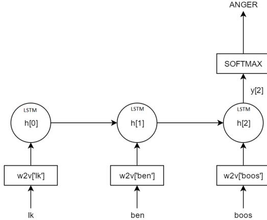
Figure 11: Diagram of the network architecture used for emotion classification.
