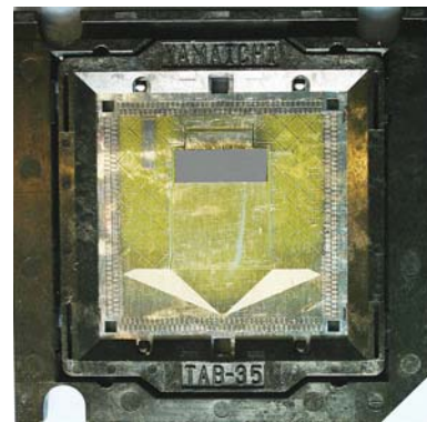
Figure 3: The framed HAL25 chip (grey rectangle) TABed on top of its chip-cable. Test pads appear along the outside of the chip-cable.
