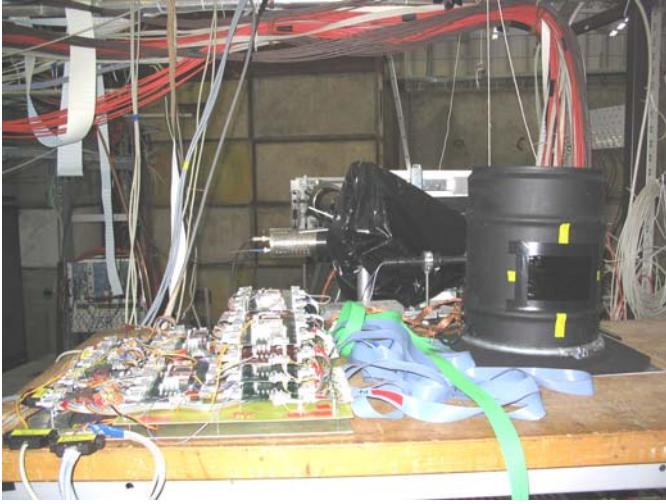
Figure 7: The beam test setup, the modules are covered by black shielding, readout is on the left and trigger in the back.
