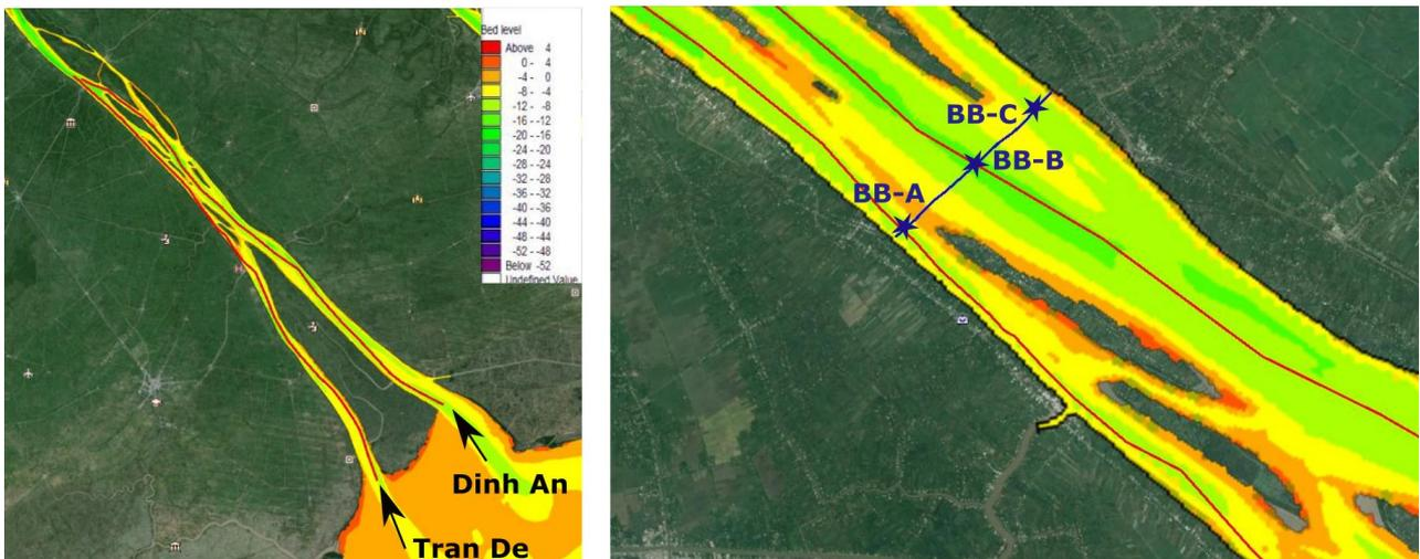
Figure 2. Along-channel transects for which salinity profiles were measured with the *moving boat* method (red trajectories in the left panel). Upstream cross section BB and locations of CTD profiles (blue stars, right panel).
