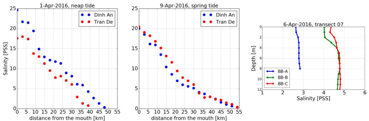
Figure 3. depth-averaged salinity along the estuary at high water slack during neap (left panel, beginning of the campaign) and spring tide (middle panel, end of the campaign). Vertical salinity profile at three locations across transect BB during ebb flow (right panel)
