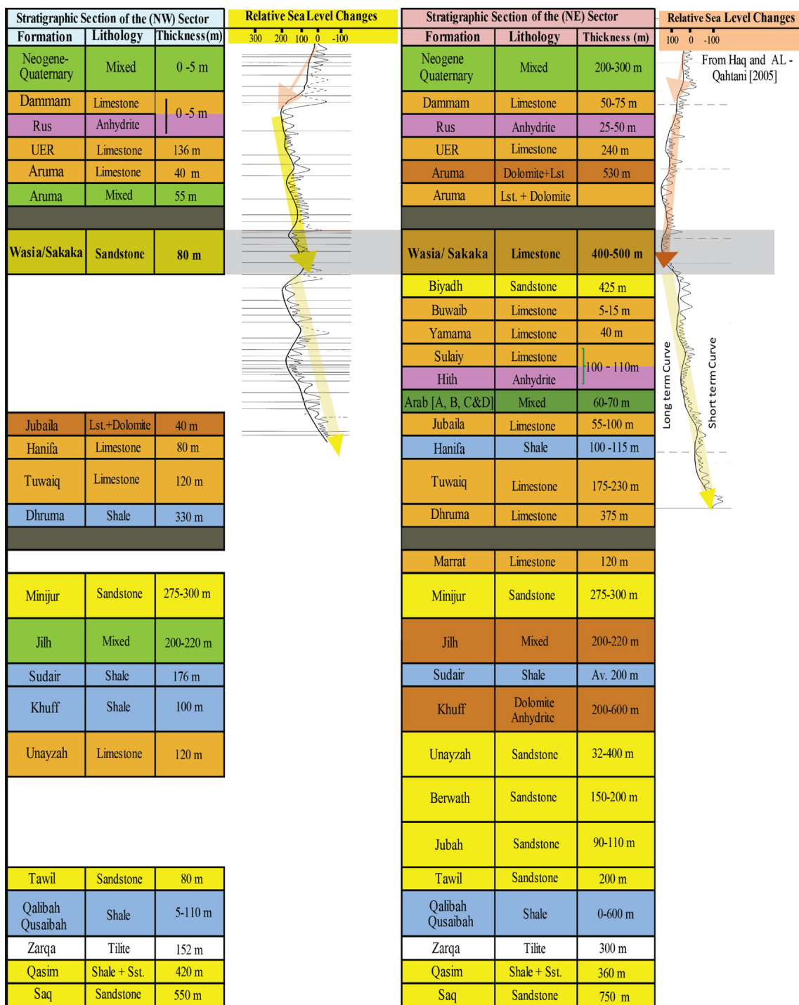
Fig. 8 Simplified stratigraphic sections and sea level variations representing the northwestern and northeastern sectors of the Arabian plate, respectively. (Modified from [Sharland et al., 2001; Haq and Al-Qahtani 2005])
