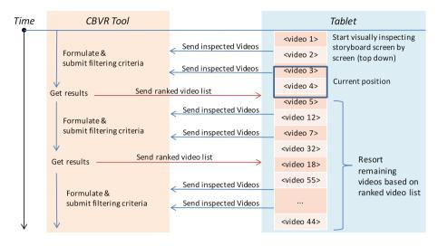
Fig. 3. Diagram explaining the collaboration between CBVR tool and tablet app.
