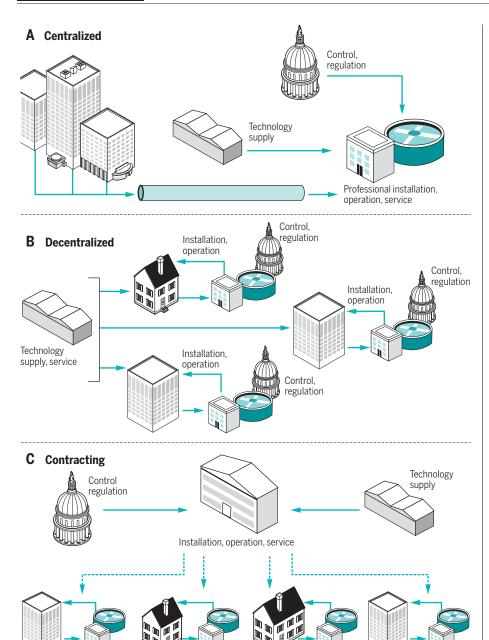
Fig. 4. Alternatives for management of centralized and decentralized wastewater treatment plants. (A) Fully centralized, (B) fully decentralized, and (C) contracting scheme for decentralized technology with centralized operation.
