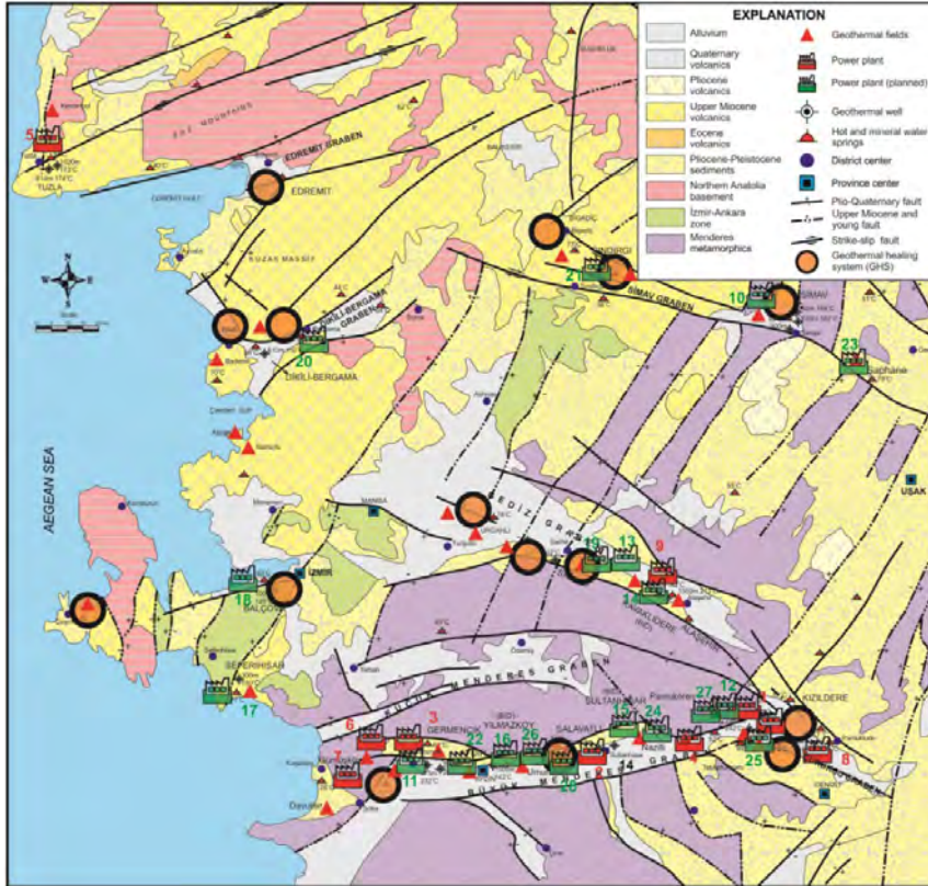
Figure 1.6: Current status of geothermal development for power generation in Western Anatolia. Modified from Mertoglu et al. [2015]. The number of the the power plants correspond to the following geothermal fields: 1. Denizli-Kızıldere, 2. Aydın-Salavatlı, 3. Aydın-Germencik, 4. Çanakkale-Tuzla, 5. Aydın-Hıdırbeyli, 6. Aydın-Gümüşköy, 7. Denizli-Geralı, 8. Manisa-Alaşehir 9. Kütahya-Simav, 10. Aydın-Germencik, 11. Denizli-Kızıldere, 12. Manisa-Alaşehir-Alkan, 13. Manisa-Alaşehir-Kavaklıdere, 14. Aydın-Sultanhisar, 15. Aydın-Yılmazköy 16. İzmir-Seferihisar, 17. İzmir-Balçova, 18. Manisa-Salihli-Caferbeyli, 19. Balıkesir-Sındırgı, 20. Aydın, 21. Kütahya-Şaphane, 22. Aydın-Nazili, 23. Aydın-Umurlu, 24. Aydın-Buharkent, 25. Aydın-Atça.
