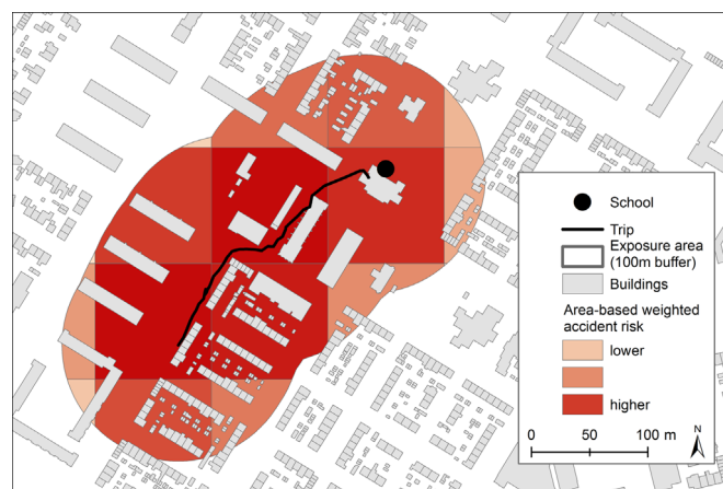
Fig. 1. Accident risk exposure along a walking trip (brighter cells receive a lower weight).
