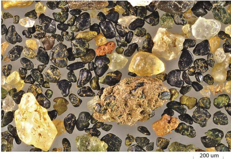
Fig. 14. Example of glauconite-rich sand illustrating the typical occurrence of this mica or clay mineral as sand-sized granules.
