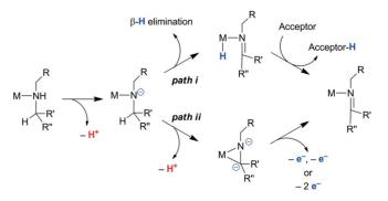
Scheme 1. Two generalized proposed pathways for imine formation via metal-amido complexes.
