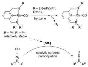
Scheme 3. Top:  $\rm H_2$  loss from a Rh-PNN amido complex. Bottom: A Rh-PNN amido complex as the catalyst for carbene carbonylation reaction to produce ketenes.  $^{[15e]}$
