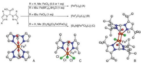
Fig. 22 Iron coordination chemistry of the substituted bispyrazolylacetato ligand family.
