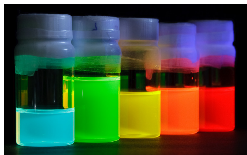
Figure 2.1 • The effect of quantum confinement on the photoluminescence of CdSe quantum dots. The vials contain colloidal dispersions of CdSe QDs with diameters ranging from 2 nm on the left to 6 nm on the right. Upon UV illumination the emission wavelength of the QDs strongly depends on their size. The colors emitted range from blue (480 nm) for the smallest QDs to red (630 nm) for the largest QDs. Photograph taken by Mark Vis.
