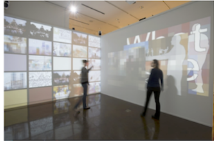
Figure 1. Specter system deployment at Time Jitters exhibit. Photo shows two people moving through the installation. Two of the four speakers are visible (top-left and center). Also visible is one of the two Kinect sensors used in the installation (top right), and one of the four projectors (each projecting to one of the four walls enclosing the installation).
