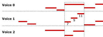
Figure 2: The baseline algorithm assigns each note to the voice having the closest reference pitch. This reference pitch is computed by averaging pitches on segments having the highest number of simultaneous notes. Here the middle voice, Voice 1, has a reference pitch that is the average of the pitches of notes 7, 9 and 11.
