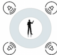
Figure 5. Migrant performance 4-channel speaker arrangement. Audience is seated in the middle. However, a regular two-speaker (stereo) setup is possible (for convenience).
