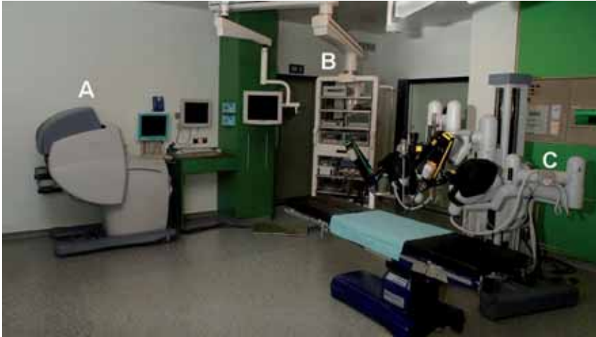
Figure 1 - The Da Vinci® surgical system consisting of the surgeon's console (A), the accessory cart (B) and the robotic surgical system (C) (see page 292 for color figure).
