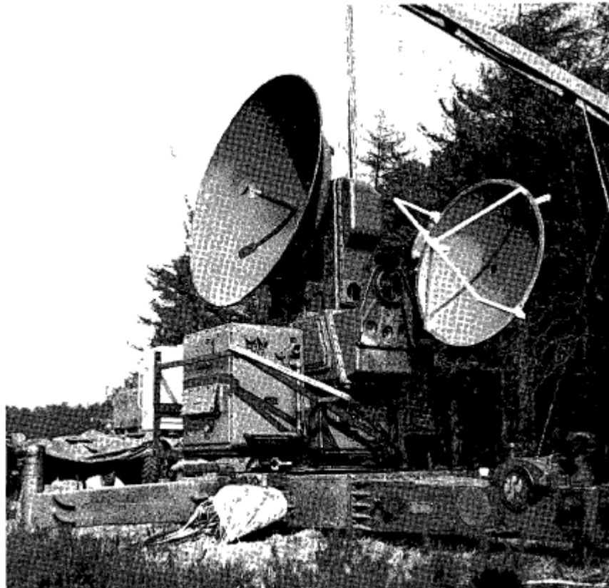
Picture 6: The measuring radar coupled with an AN/MPQ-10 tracking radar Fysisch laboratorium 1927-1977, J.L. van Soest
