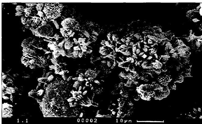
Photo 3 Synthetic zeolite Na-P1 (synthesized from fly ash)
