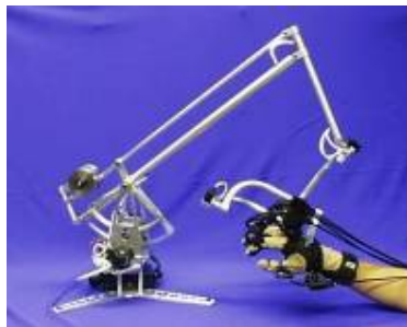
Figure 2 Example of Exoskeleton [17] : These devices are less disseminated than the previous class, but they offer a much higher level of realism
