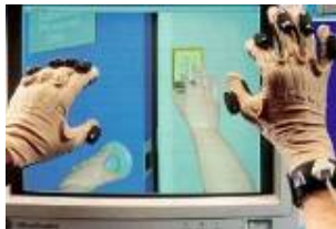
Figure 3 Tactile display [18]: These devices aren't force feedback but rather tactile feedback devices i.e. they give the sense of touch: shape,
