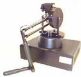
Figure 1 The Arm-like Device [16] : The user grasp a robotic arm with several degrees of freedom that can apply forces.
