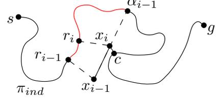
**Figure 2:** Only the subpath of  $\pi_{ind}$  between  $r_{i-1}$  and  $\alpha_{i-1}$  (shown in red) is taken into consideration for the computation of reference point  $r_i$ . Choosing the closest point  $c$  as the reference point would lead to an undesired shortcut.
