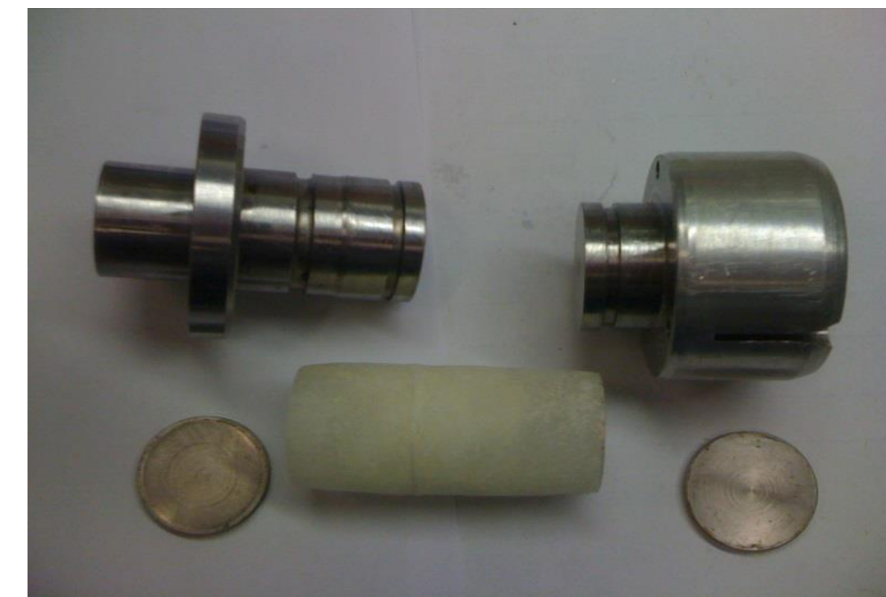
Figure 1. Bischofite sample with piston assembly
