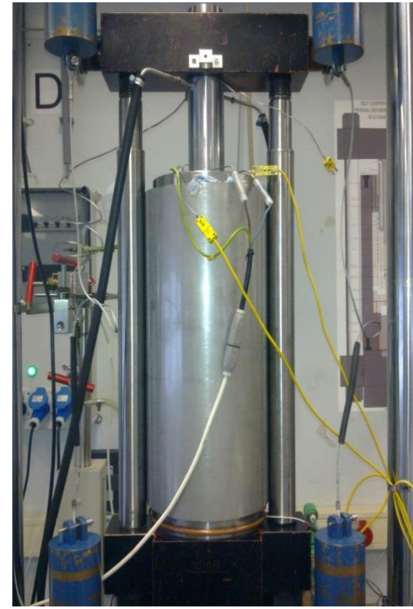
Figure 3. Triaxial apparatus (Shuttle vessel)
