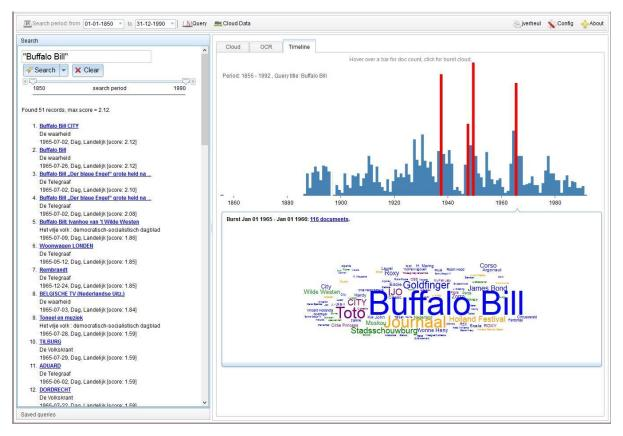
Fig. 3: Result of a query with a timeline and word cloud based on one 'burst' (indicated in red); the named entities in the word cloud are indicated by colors
