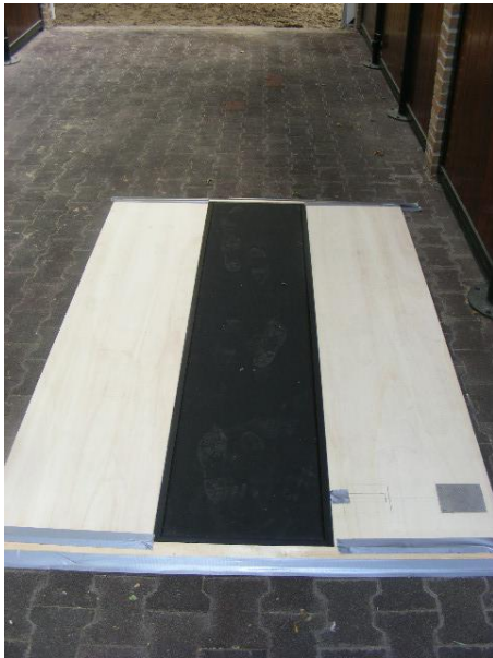
Figure 1: The setting of the pressure plate without the rubber mat.
