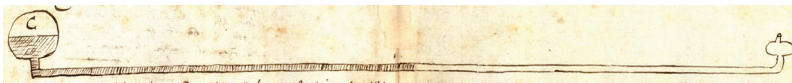
Fig. 6: Reneri's horizontal version of the reversed two-bulbed thermometer in his letter to Huygens of 22 October 1635 (courtesy of Uppsala Universitetsbibliotek).
