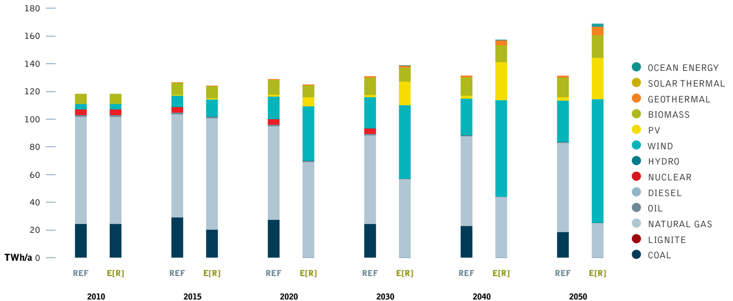
figure 5.5: electricity generation structure under the reference scenario and the energy [r]evolution scenario (INCLUDING ELECTRICITY FOR ELECTROMOBILITY, HEAT PUMPS AND HYDROGEN GENERATION)
