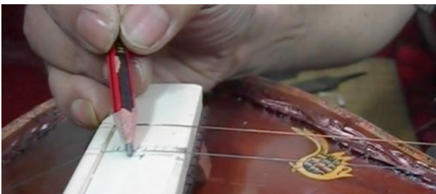
Figure 3. Sitar Maker Barun Roy shows the location of the area to file in order to close the main strings’ jawari on an unfinished sitar (Kolkata, 11 April 2011. Photo: S. Weisser).
