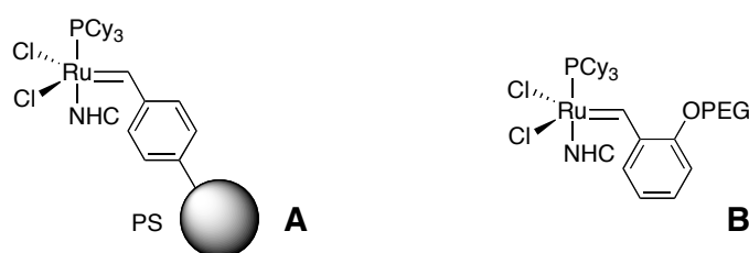
Figure 30. a) Polystyrene bound ruthenium benzylidene complex; b) PEG bound benzylidene complex.
