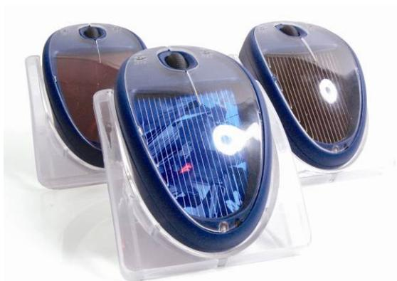
**Figure 2:** Photographs of three SPM prototypes each equipped with a different solar cell type
