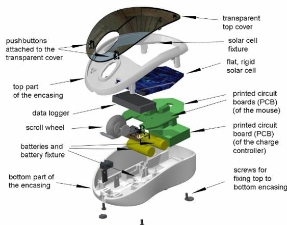
**Figure 1:** Final design concept of the SPM prototypes
