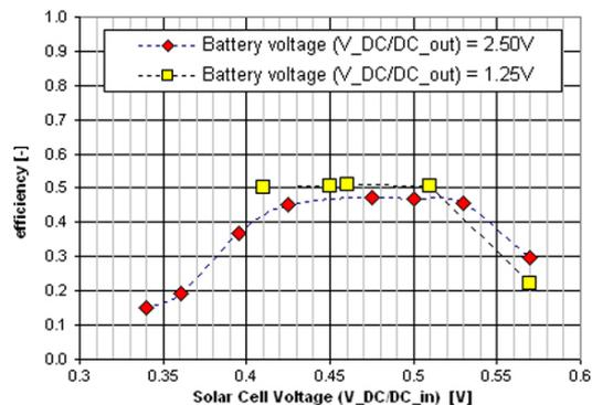
**Figure 4:** Very low voltage conversion efficiency (max. 50%) of the first voltage conversion unit
