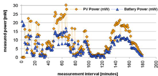
**Figure 6:** PV and battery power measured for 3 hours of a SPM located at a desk at TU Delft, The Netherlands
