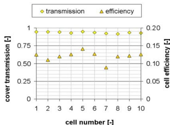
**Figure 3:** Measured transmission of the transparent cover and efficiency of the (mono and multi) crystalline silicon solar cells.
