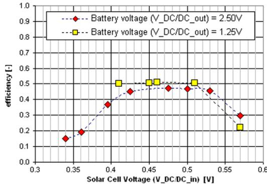
**Figure 4:** Very low voltage conversion efficiency (max. 50%) of the first voltage conversion unit
