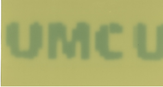
Figure 4.17: IMRT fields delivered on the MRI-linac prototype, that together form the acronym UMCU. The radiation fields were recorded on GafChromic EBT2 radiation sensitive film.
