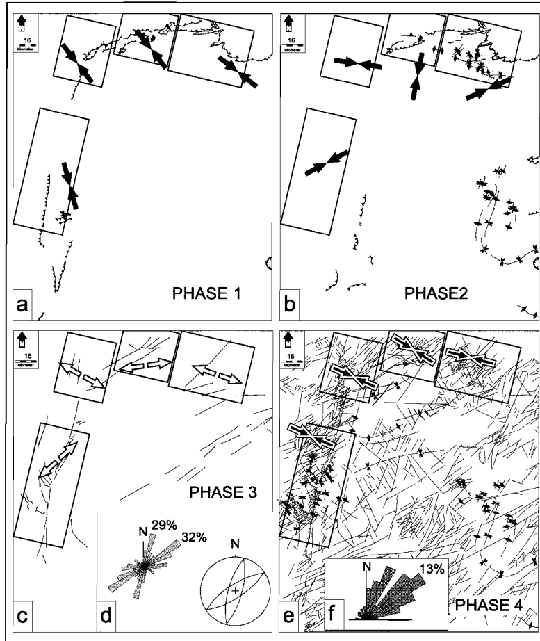
Figure 5.11 Plots of the horizontal components of the \sigma_1 for phases-1, 2 and 4 (converging large arrows) and the \sigma_3 for the phase-3 (diverging large arrows) and the structures proposed to have been developed in the corresponding phase (a,b,c and e). d) Length weighted rose diagram prepared from the faults that proposed to have been developed in the deformation phase-3 and idealized stereographic projection of largest populations note that they display 2 sets of conjugate fault pairs. f) Length weighted rose diagram prepared from the faults proposed be have been developed in the deformation phase-4.
