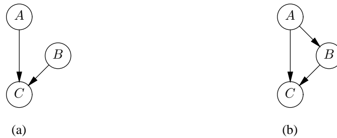
Figure 8.2: The graphical parts of two small example Bayesian networks, one of which is singly connected (a) and one of which is multiple connected (b).
